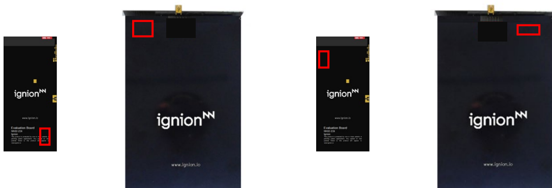
Figure 3 – Placement of the connection pins on the connectivity board (from left to right: set-up 1 (corner long edge), set-up 2 (corner short edge)).
